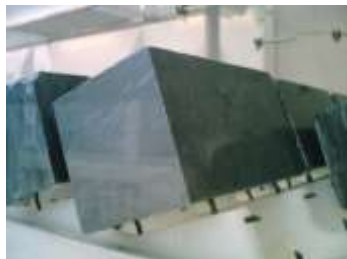
Close-up of typical silicon blocks being processed
